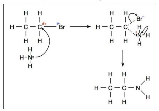
The intermediate formed has an N<sup>+</sup> atom, so electrons are transferred to it causing a hydrogen to be lost.
